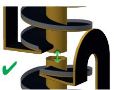
The J-Configuration is unique as it does NOT require such straight segment and by that, it is easily stackable. The upper end of the lower spiral can be connected to the lower end of the upper spiral in one ongoing helical flow.
