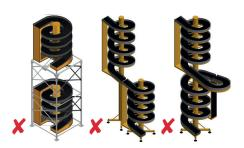
Because of the straight section spiral conveyors cannot be stacked in one line but need loops or an offset stack. Such solutions interrupt the continuous flow, add cost and consume space.
