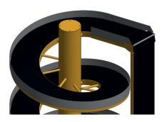
Spiral conveyors are known to elevate over multiple windings with one belt returning straight down to the lower end. This return requires a straight section on the upper end of the spiral to reach out of the spiral circle.
